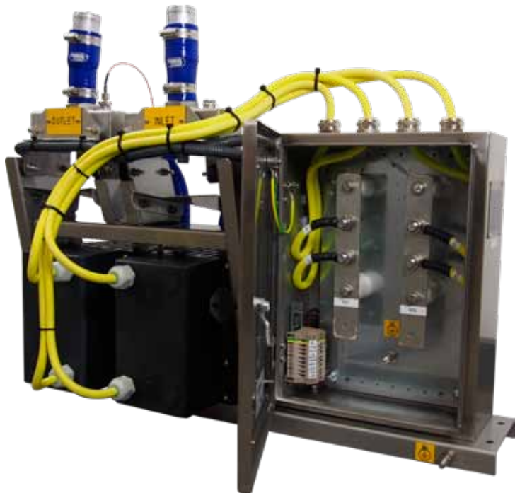
EV2 resistors used to control hoists on board ship. The open back plate assembly holds 2 x 4EV2 assemblies to give a maximum continuous power of 200kW.
