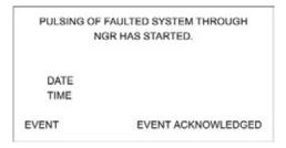
This screen is displayed when the viewed event record in the "Events" data table is for the initiation of the NGR pulse. The "Event Acknowledged" tag is only displayed when the user has previously pressed the "ACK ALARM" key. Pressing "ESC/BACK" will return the user to the "View Alarms Events" screen.
