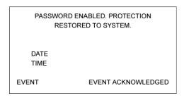
This screen is displayed when the viewed event record in the "Events" data table is for the re-activation of the password function. The "Event Acknowledged" tag is only displayed when the user has previously pressed the "ACK ALARM" key. Pressing "ESC/BACK" will return the user to the "View Alarms Events" screen.
