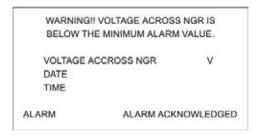
This screen is displayed when the viewed alarm record (code 12) in the "Alarms" data table is an NGR undervoltage condition. The "Alarm Acknowledged" tag is only displayed when the user has previously pressed the "ACK ALARM" key. Pressing "ESC/BACK" will return the user to the "View Alarms Events" screen.
