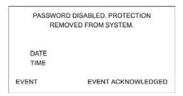
This screen is displayed when the viewed event record in the "Events" data table is for the disabling of the password function. The "Event Acknowledged" tag is only displayed when the user has previously pressed the "ACK ALARM" key. Pressing "ESC/BACK" will return the user to the "View Alarms Events" screen.
