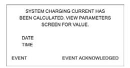
This screen is displayed when the viewed event record in the "Events" data table is for the calculation of the system charging current. The "Event Acknowledged" tag is only displayed when the user has previously pressed the "ACK ALARM" key. Pressing "ESC/BACK" will return the user to the "View Alarms Events" screen.
