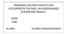
This screen is displayed when the viewed alarm record (code 113) in the "Alarms" data table is an NGR opencircuit failure condition. The "Alarm Acknowledged" tag is only displayed when the user has previously pressed the "ACK ALARM" key. Pressing "ESC/BACK" will return the user to the "View Alarms Events" screen.
