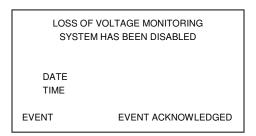
This screen is displayed when the viewed event record in the "Events" data table is for the disabling of the loss of voltage function. The "Event Acknowledged" tag is only displayed when the user has previously pressed the "ACK ALARM" key. Pressing "ESC/BACK" will return the user to the "View Alarms Events" screen.
