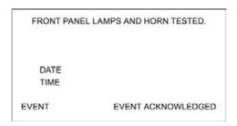
This screen is displayed when the viewed event record in the "Events" data table is for the testing of the front panel lamps and alarm horn. The "Event Acknowledged" tag is only displayed when the user has previously pressed the "ACK ALARM" key. Pressing "ESC/BACK" will return the user to the "View Alarms Events" screen.
