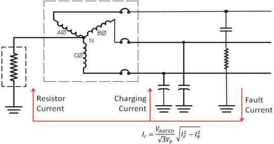
Where: V<sub>RATED</sub> = System Voltage taken from System Values Screen
