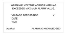
This screen is displayed when the viewed alarm record (code 11) in the "Alarms" data table is an NGR overvoltage condition. The "Alarm Acknowledged" tag is only displayed when the user has previously pressed the "ACK ALARM" key. Pressing "ESC/BACK" will return the user to the "View Alarms Events" screen.
