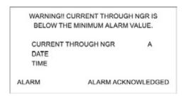
This screen is displayed when the viewed alarm record (code 22) in the "Alarms" data table is an NGR undercurrent condition. The current through the NGR in amps and the date and time of the alarm are displayed. The "Alarm Acknowledged" tag is only displayed when the user has previously pressed the "ACK ALARM" key. Pressing "ESC/BACK" will return the user to the "View Alarms Events" screen.
