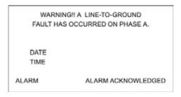
This screen is displayed when the viewed alarm record (code 71) in the "Alarms" data table is a single-line-toground fault detected by the phase A voltage monitoring relay. The "Alarm Acknowledged" tag is only displayed when the user has previously pressed the "ACK ALARM" key. Pressing "ESC/BACK" will return the user to the "View Alarms Events" screen.
