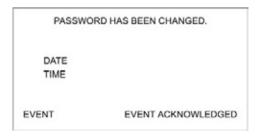
This screen is displayed when the viewed event record in the "Events" data table is for the changing of the customer password. The "Event Acknowledged" tag is only displayed when the user has previously pressed the "ACK ALARM" key. Pressing "ESC/BACK" will return the user to the "View Alarms Events" screen.
