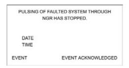
This screen is displayed when the viewed event record in the "Events" data table is for the termination of the NGR pulse. The "Event Acknowledged" tag is only displayed when the user has previously pressed the "ACK ALARM" key. Pressing "ESC/BACK" will return the user to the "View Alarms Events" screen.
