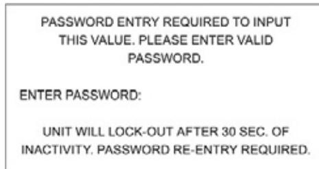
This screen is used for entry of the customer password. It is accessed by pressing the “EDIT” key on the front panel. Once the password has been successfully entered, the user will be returned to the previous screen. The default password is 1000.
