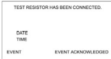
This screen is displayed when the viewed event record in the “Events” data table is for the connection of the test resistor. The “Event Acknowledged” tag is only displayed when the user has previously pressed the “ACK ALARM” key. Pressing “ESC/BACK” will return the user to the “View Alarms Events” screen.
