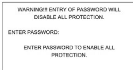
This screen is accessed by pressing the “F2” key on the “Password Extras” screen. On this screen, entry of the customer password will disable the password function. When the password is active, the text above the entry box displays. When the password is disabled, the text below the entry box displays. To enable the password, the user enters the customer password. Pressing “ESC/BACK” will return the user to the “Password Extras” screen.
