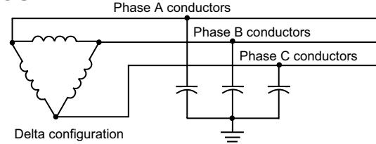
the normal voltage is present on all insulation in the system, as shown in Figure 3b. This situation can often cause failures in older motors and transformers, due to insulation breakdown.
