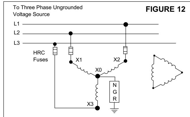
The transformer primary voltage rating should be equal to or greater than the line-to-line voltage of the system to which it is being connected.
