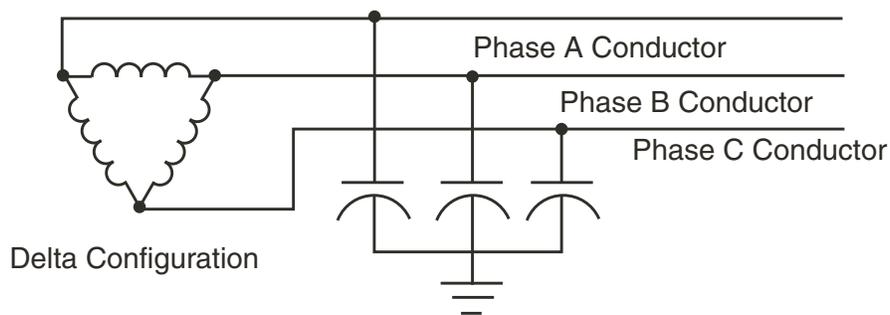
Under normal operating conditions this distributed capacitance causes no problems. In fact, it is beneficial because it establishes, in effect, a neutral point for the system, as shown in Figure 3a. As a result, the phase conductors are stressed at only line-to-neutral voltage above ground.
