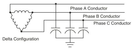
Under normal operating conditions this distributed capacitance causes no problems. In fact, it is beneficial because it establishes, in effect, a neutral point for the system, as shown in Figure 3a. As a result, the phase conductors are stressed at only line-to-neutral voltage above ground.
