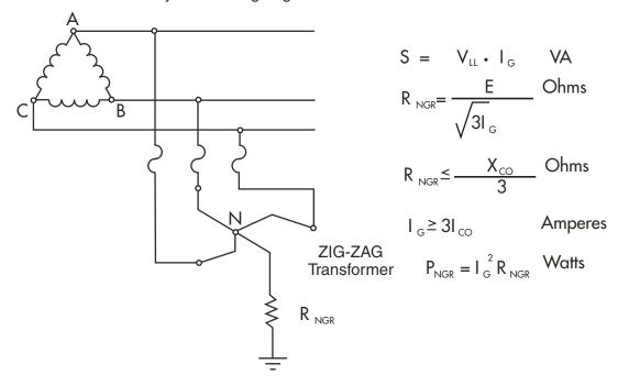
With pre-packaged High Resistance Grounding Systems available from Post Glover, all with enclosed current limiting Neutral Grounding Resistors and artificial neutrals, the process is to determine the protective features that you require and install the product of choice.
