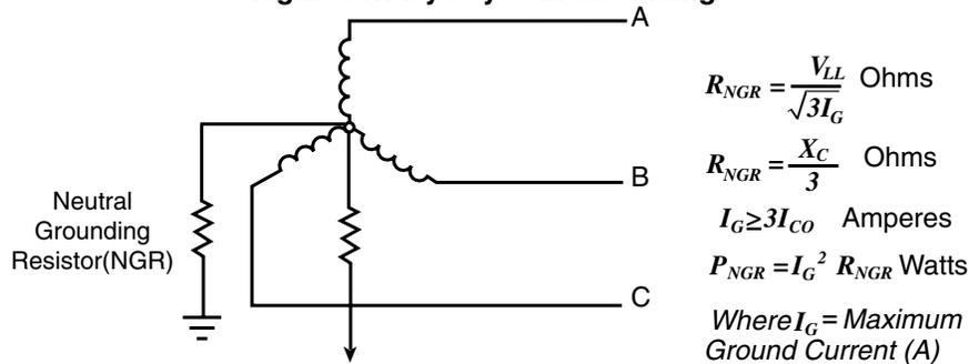
**Figure 3.2: Medium-voltage Wye System Grounding**
