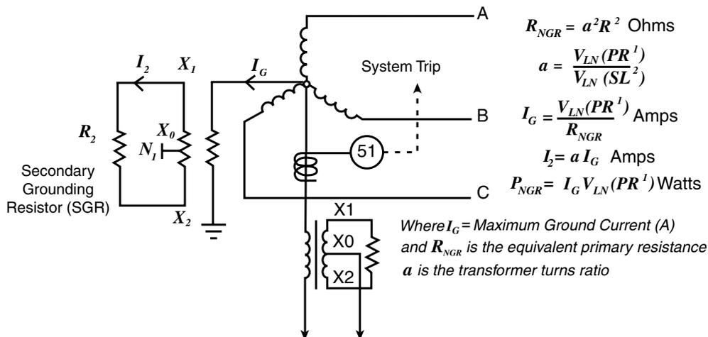
**Figure 3.3: Delta System Grounding**
