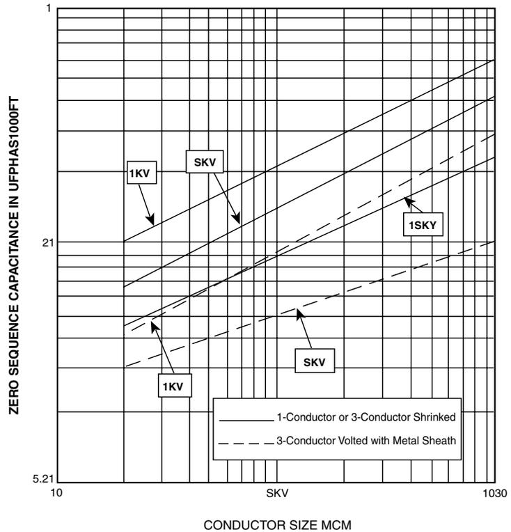
Figure A1.3: Motor Capacitance to Ground Values
