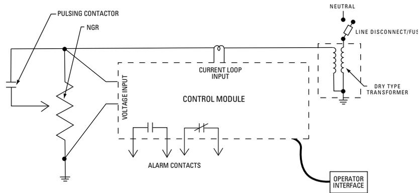
Figure 8.2 (b) Pulser Plus Wye-Connected Medium Voltage Pulse System
