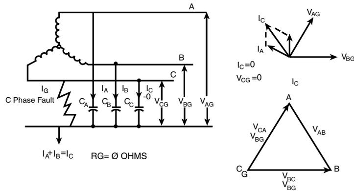
Even though the capacitive voltages are unequal during a single line-to-ground fault, the phase-to-phase voltages ( $V_{AB}$ ,  $V_{AC}$  and  $V_{BC}$ ) have not changed in magnitude or phase relationship and the system remains in service. Ground Current in the fault  $I_G$  is the vector sum of the two currents  $I_A$ , and  $I_B$ , (which are  $90^\circ$  ahead of their respective voltages  $V_{AG}$  and  $V_{BG}$ ) where  $I_A = V_{AG}/X_A$  and  $I_B = V_{BG}/X_B$ .
