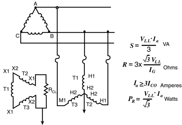
**Figure 3.4: Delta System Grounding For Medium Voltage**
