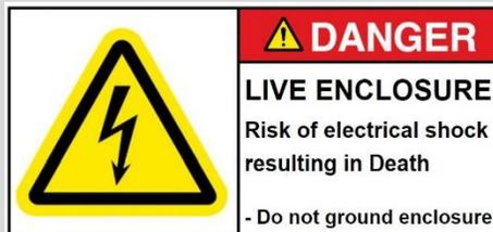
Only if the enclosure is not tied to center potential should the enclosure be grounded (to prevent a shock hazard to personnel or wildlife). The product specific drawing will state whether the enclosure is tied live.
