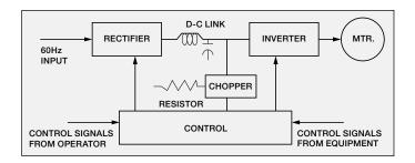
A three-phase variable frequency drive (VFD) consists of three basic components – rectifier, DC line, and inverter. The rectifier converts the
