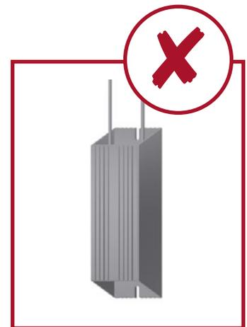
**WARNING: Do not mount unit with leads pointing upwards.**
