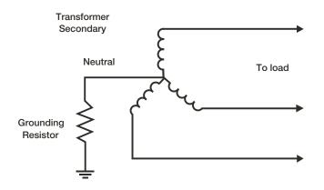
The reason for limiting the current by resistance grounding may be one or more of the following, as indicated in IEEE Std. 142-1991, IEEE Recommended Practice for Grounding of Industrial and Commercial Power Systems, Section 1.4.3.
