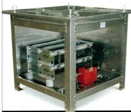
Neutral grounding resistors are used for resistance grounding of industrial power systems. They are designed to limit the maximum fault current to a value that will not damage generating, distribution or other associated equipment in the power system.
